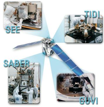
SABER (Sounding of the Atmosphere using Broadband Emission Radiometry)—A multi-channel infrared radiometer designed to measure heat emitted by the atmosphere over a broad altitude and spectral range. SABER will also measure global temperature profiles and sources of atmospheric cooling, such as the "air glow," which occurs when energy is radiated back into space.
