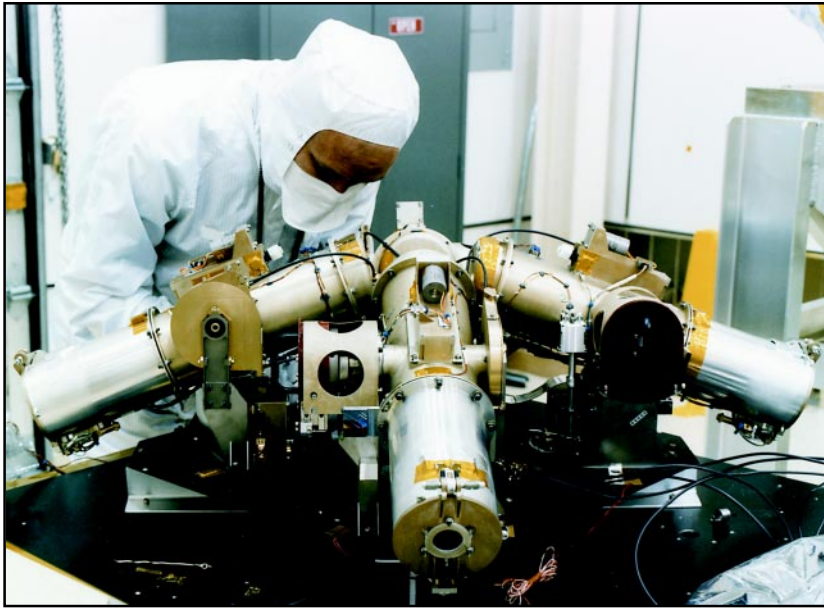
TIDI's telescopes are prepared for placement onto the spacecraft.
